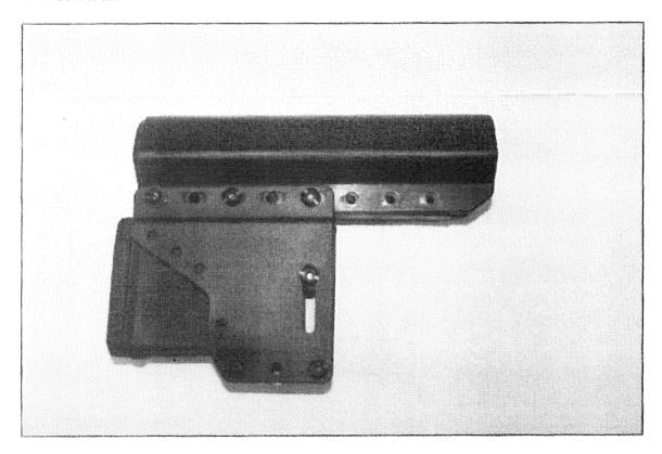
After a phone conversation with Mr. Vasquez, you have redesigned your submission by removing the two rearward holes to limit travel. Additionally, you have redesigned the magazine storage device to hold the magazine vertical instead of horizontal.
